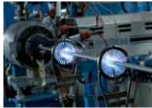
PE-X and composite pipe fabrication
