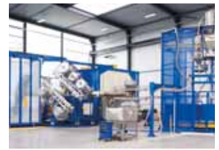
Rotation plant for grease separators
